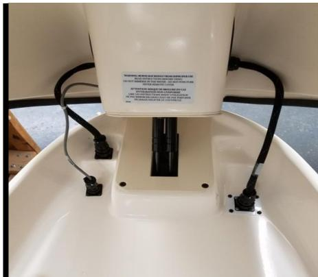
Figure 7.1.1 Releasing Electrical Connectors.
