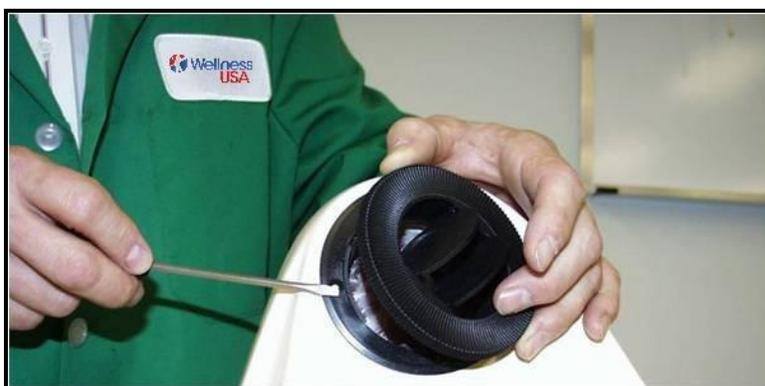
**Figure 7.16.1 Removing Face Air Vent(s).**
