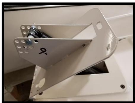
**Figure 7.4.1 Pin Bolt on Upper Hinge Assembly**
