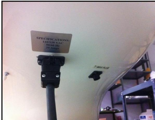
Figure 4.7.1 Connection of Power Cord.
